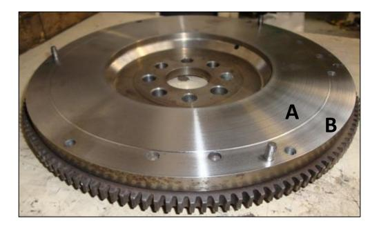
M40 Minimum of 22.7mm on the inner surface. (Point A)Minimum of 44.5mm on the outer surface. (Point B)Minimum weight of 9.00kg, including 3 dowels but no mounting bolts.
